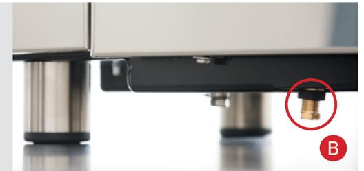
9. Should the pump pressure require adjusting, it is externally adjustable from under the machine (Fig B). With care using a 14mm socket loosen the pump pressure adjustment lock ring.
